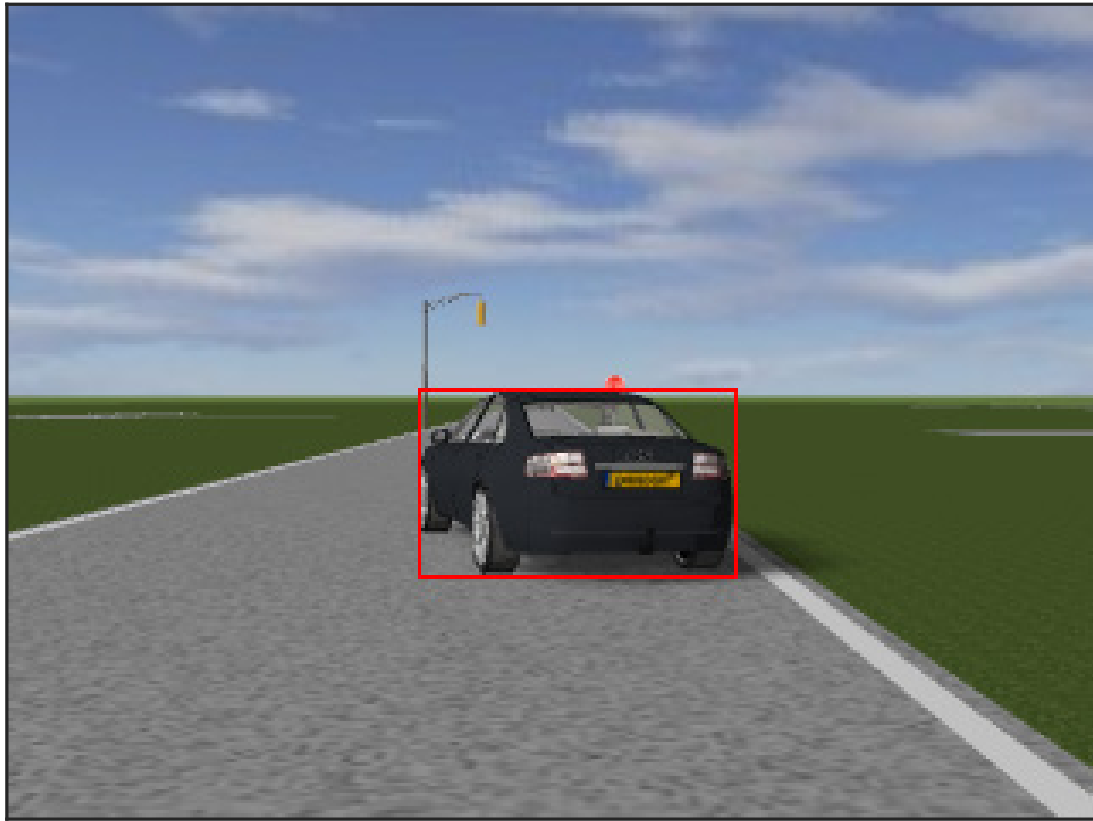
Figure 4.4: Object detected in the path of the ego vehicle through the vision sensor
